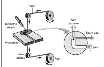
Fig. 13.4.21 Schematic diagram of the wire EDM process.
