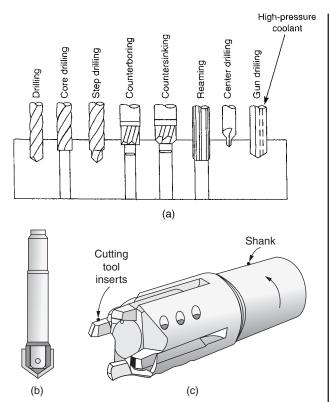
**Fig. 13.4.14** (*a*) Various types of drills and drilling and reaming operations; (*b*) spade drill; (*c*) trepanning tool with four cutting-tool inserts.
