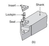
Fig. 13.4.8 (a) Insert clamped to shank of a toolholder; (b) insert clamped with wing lockpins.
