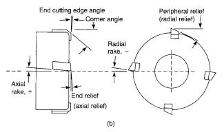
Fig. 13.4.16 (a) Plain milling cutter teeth; (b) face milling cutter.
