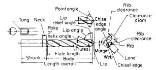
Fig. 13.4.13 Straight shank twist drill.
