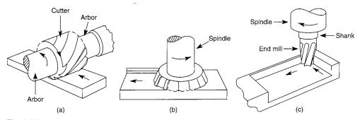
Fig. 13.4.15 Basic types of milling cutters and operations. (a) Peripheral milling; (b) face milling; (c) end milling.
