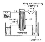
Fig. 13.4.22 Schematic diagram of the electrochemical machining process.
