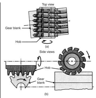
Fig. 13.4.17 A gear-cutting hob.
