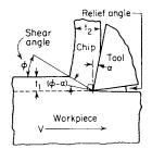
Fig. 13.4.2 Basic mechanics of metal cutting process.
