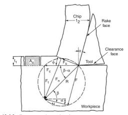
Fig. 13.4.3 Force system in metal cutting process.
