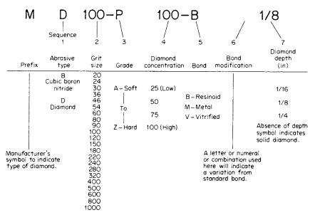
Fig. 13.4.19 Standard marking system chart for diamond tool and cubic boron nitride (cBN) bonded abrasives.
