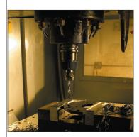
With plastics, always consider heat tolerances and keep in mind that drilling generates more heat than any other machining technique.
